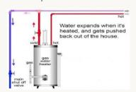
Many things can cause issues with a T&P valve. For example, the constant dripping of water can cause natural mineral deposits to occur creating a blockage, causing the T&P valve to become ineffective. If the water temperature increases to more than 212 °F (111 °C) the tank is
