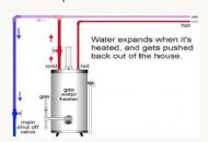
Many things can cause issues with a T&P valve. For example, the constant dripping of water can cause natural mineral deposits to occur creating a blockage, causing the T&P valve to become ineffective. If the water temperature increases to more than 212 °F (111 °C) the tank is considered
