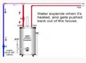
Many things can cause issues with a T&P valve. For example, the constant dripping of water can cause natural mineral deposits to occur creating a blockage, causing the T&P valve to become ineffective. If the water temperature increases to more than 212 °F (111 °C) the tank is considered
