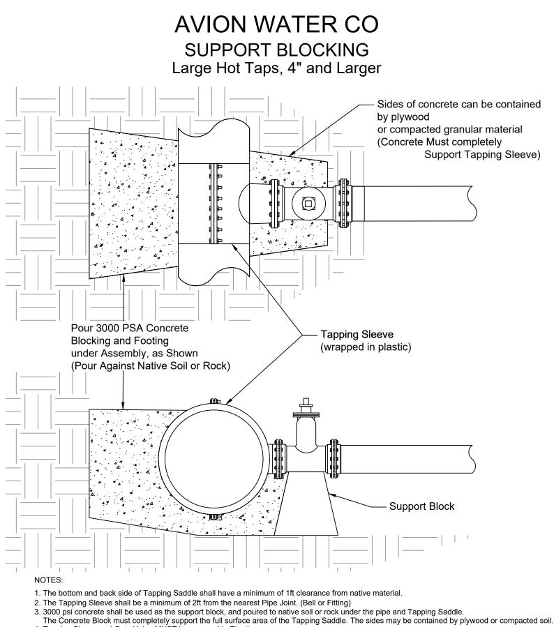
4. Tapping Sleeve and Gate Valve MUST be wrapped in Plastic.
