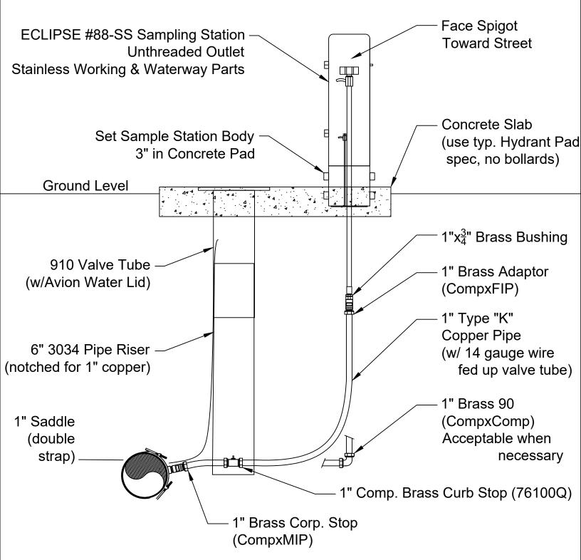
ALL PIPE AND CONCRETE PAD SHALL BE BACKFILLED WITH COMPACTED  $\frac{3}{4}$ "-0, OR EQUIVALENT
