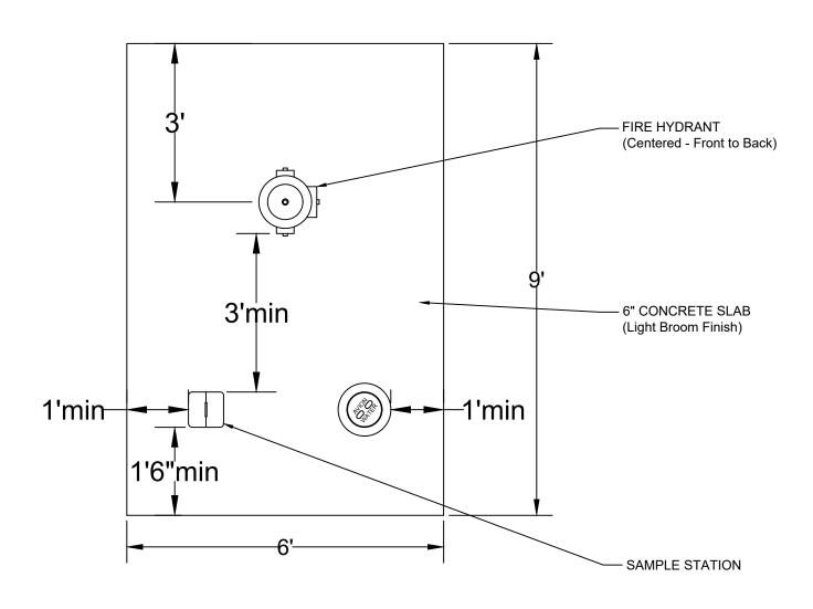
ALL PIPE AND HYDRANT PAD SHALL BE BACKFILLED WITH COMPACTED 3/4"-0, OR EQUIVALENT
