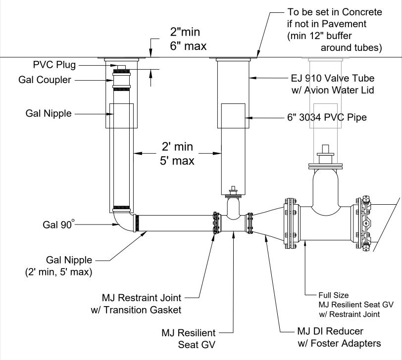
Match all fitting sizes with size of Blow Off called out in plans.
