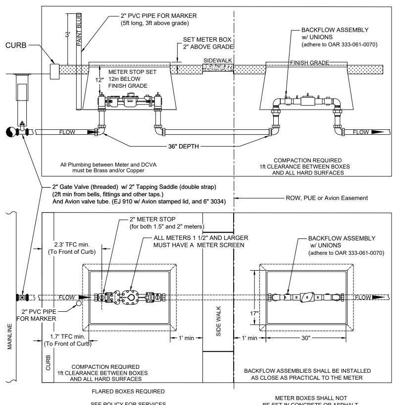
SEE POLICY FOR SERVICES FOR METER/BPA BOX AND LID SPECIFICATIONS BE SET IN CONCRETE OR ASPHALT
